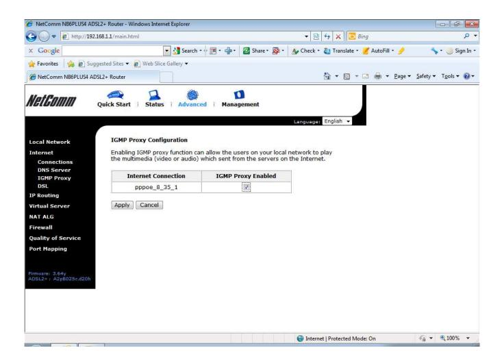
4. Check to enable the **IGMP proxy** and press Apply.
