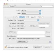
13. If your Mac does not accept an IP address from the DHCP server in your NBWMAXX and the IP address field remains blank, try selecting "Using DHCP with manual address" from the "Configure iPV4" pop-up menu and entering 192.168.1.3 in the "IP address" field.
