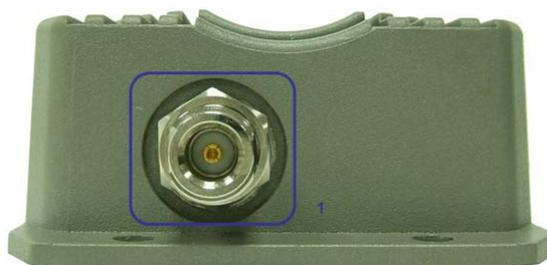
1. N-type Connector: For connection to antenna.
