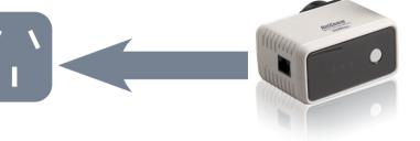
4. Connect the second Powerline Adapter to a wall power socket
