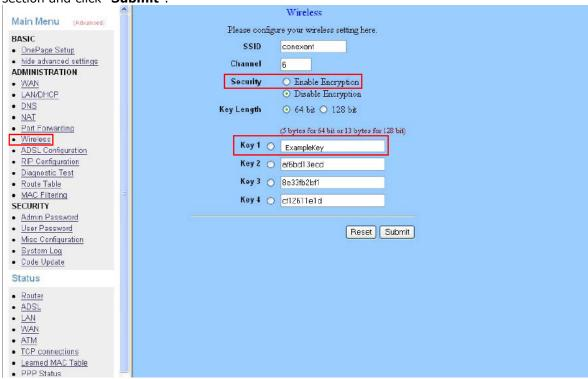
Any changes to your wireless security settings will require you to reconfigure any wirelessly connected devices to use the new security settings. This is done by removing any stored wireless settings and then reconnecting to your wireless network.
