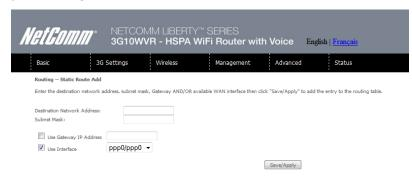
Enter Destination Network Address, Subnet Mask, Gateway IP Address and/or WAN Interface. Then click Save/Apply to add the entry to the routing table.
