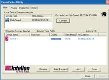
The Set Local Device Only button is used to change the network name (network password) for the local device only. After doing this, all the devices seen on the Main panel prior to this will no longer be able to communicate or respond to the computer, as they will be on a different logical network. Devices previously set up with the same logical network (same network name) will appear in the device list afterward selecting this option.
