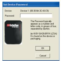
A dialog box will appear as shown below to type the password. The selected device name is shown above the field for entering the password.
