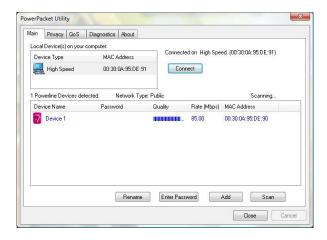
The top panel shows all local Powerline devices found connected to the computer's NIC (Network Interface Card). In most cases, only one device will be seen. In situations where there are more than one device connected, such as a USB and also an Ethernet device, the user may click to select the one to manage through and then click the Connect button to its right. The status area above the button indicates that your PC is connected to that same device.
