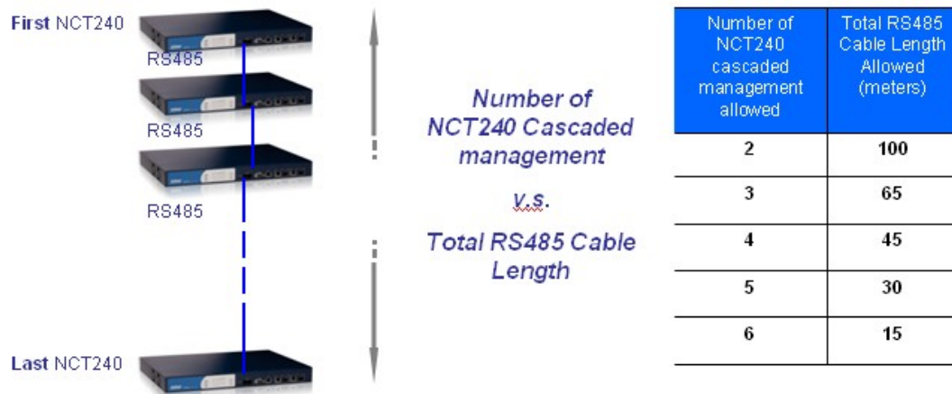
Figure 3: RS485 total cable length vs number of Daisy Control NCT240 IP DSLAMs allowed
