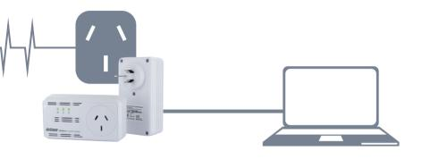
Connect one end of the other supplied Ethernet cable into the Ethernet port of any device you want to connect to the Internet (PC, set-top box, gaming console, PVR, blu-ray player etc).
