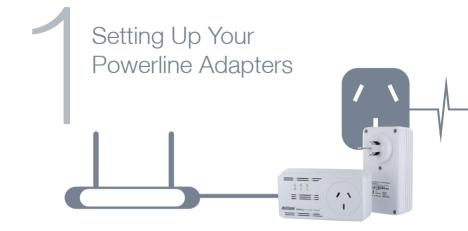
Using one of the supplied Ethernet cables connect one end into the LAN Ethernet port of your modem/router.
