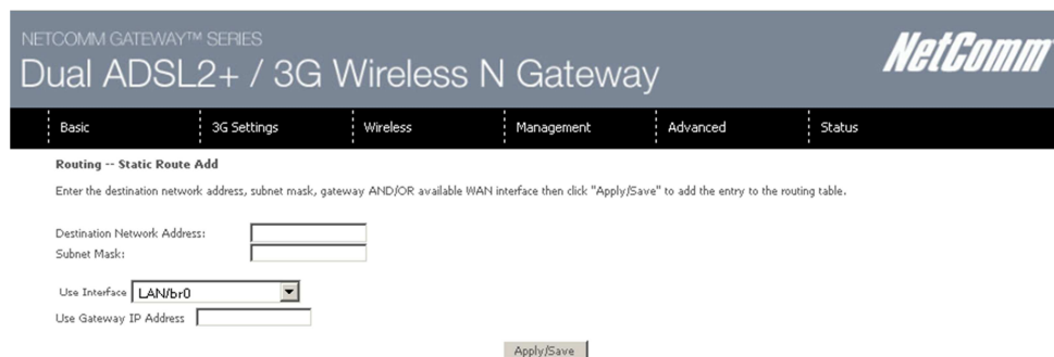
Figure 56: Advanced - Routing - Add Static Route
