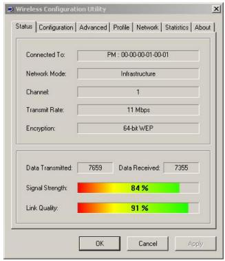
The lower section of the dialog box shows the data transmitted and received; the two signal lines show the Signal Strength and the Link Quality of the device.
