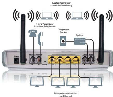
You can connect multiple wireless devices, including laptops, desktops and PDA's to your NB9WMAXXn by following the 2 basic steps
