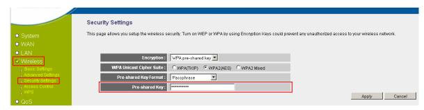
If you would like to select a different network security type instead, click the drop down menu in the "**Encryption**" section and select the desired security type.
