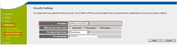
4. After selecting your desired security type (we're using WPA2-PSK for the example), enter the wireless security key you would like to use into the "WPA Pre-Shared Key:" section and click "Apply".
