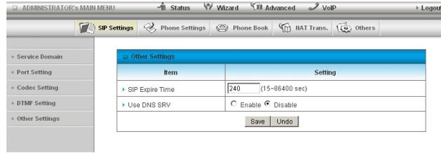
The Other Settings page enables you to specify a different SIP expire time and select to enable the DNS SRV function. This information will usually be supplied by your VOIP service provider and should not need to be changed unless you are experiencing issues with VOIP calls or signing into your VOIP service.
