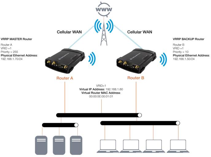
Figure 2 - VRRP in Action - How it operates on Ethernet
