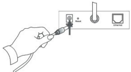
**TIP:** You can confirm power source is supplied from the LED indicators label Power on the Pan/Tilt Internet Camera is illuminated.
