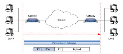
IPSec uses the Internet Key Exchange (IKE) protocol to facilitate and automate the SA setup and the exchange of keys between parties transferring data. IPSec requires that keys be recreated, or refreshed, frequently so that the parties can communicate securely with each other. IKE manages the process of refreshing keys; however, a user can control the key strength and the refresh frequency. Refreshing keys on a regular basis ensures data confidentiality between sender and receiver.
