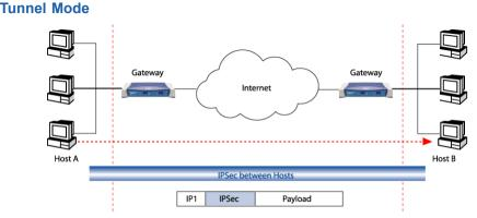
The tunnel mode IPSec implementation encapsulates the entire IP packet.
