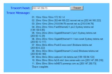
Note: Not all routers in an IP path will allow self identification hence you may see some hops along the way left as blanks. Also it is possible that the final destination may not respond to the Trace Route Query even though it exists and can exchange data via TCP / IP.
