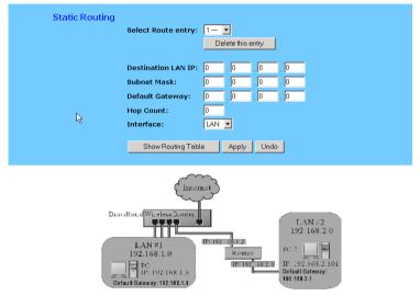
In the above diagram, PC2 in LAN#2 is connected to the NetComm Cable/DSL Firewall Router via another router while PC1 in LAN#1 is connected to the NetComm Cable/DSL Firewall Router directly. Without configuring the Static Routing function, the two computers would not be able to communicate with each other.
