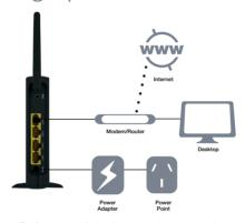
Take the **Wireless Access Point** out of the box and connect it to your broadband modem/router with one of the supplied Ethernet cables.
