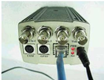
**Note:** Ensure you power supply adapter specification. NS4120 uses a 'DC 12V 1A' power supply. NS4000/4100/4240 use a 'AC 14V/13.8V 1A' power supply. The Input AC Voltage must match to your power system, e.g. 110V/220V.
