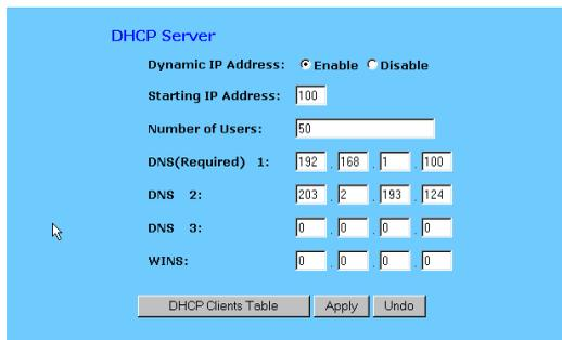
**Note:** The DHCP Server can support a maximum pool of 253 IP Addresses.
