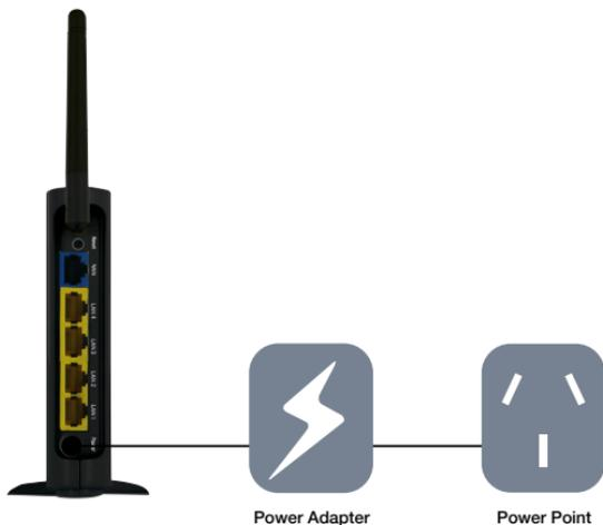
4. Connect the supplied **power adapter** to the **Power socket** at the back of your **Wireless N Router**
