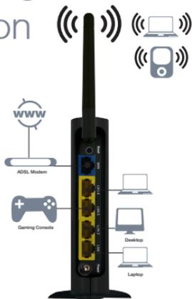
You can connect multiple wireless devices, including laptops, desktops and PDA's to your **Wireless N Router** by following these two basic steps.
