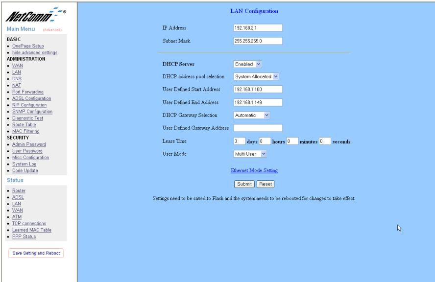
**LAN IP Address & Subnet Mask:** The default is 192.168.1.1 and 255.255.255.0 you can change it to another private IP address, such as 172.168.0.1, and 255.255.255.0. - For most configurations it is recommended to leave it as default.
