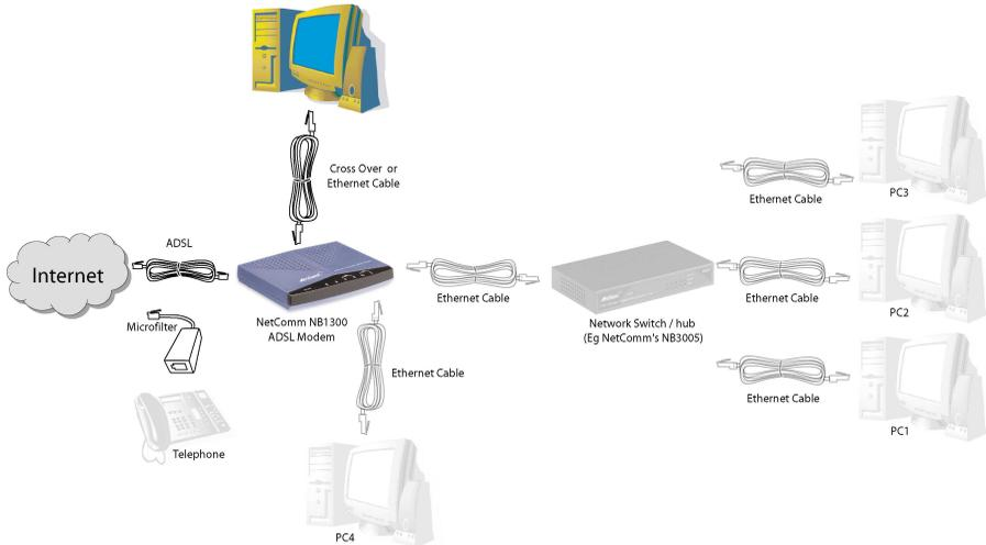
**Ethernet Gateway** (performing Network Address Port Translation) - This is when the NB1300 is connected to your network switch or hub and shares the Internet connection to all computers on the network. The NB1300 will log on to your ISP on behalf of your computers and it will shield your computers from direct Internet attack by using Network address Translation (NAT).
