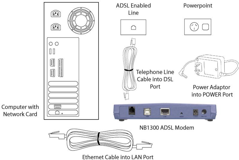
2. Connect the power pack to the NB1300 ADSL Modem and switch on the power switch.
