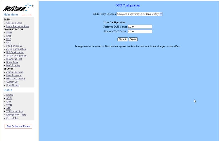
**Disable DNS Proxy:** The LAN port does not process the DNS query message. For the DHCP requests from local PCs, the DHCP server will set the user-configured preferred DNS server or alternate DNS server whichever is available as the DNS server. Then all DNS query messages will be directly sent to the DNS servers.
