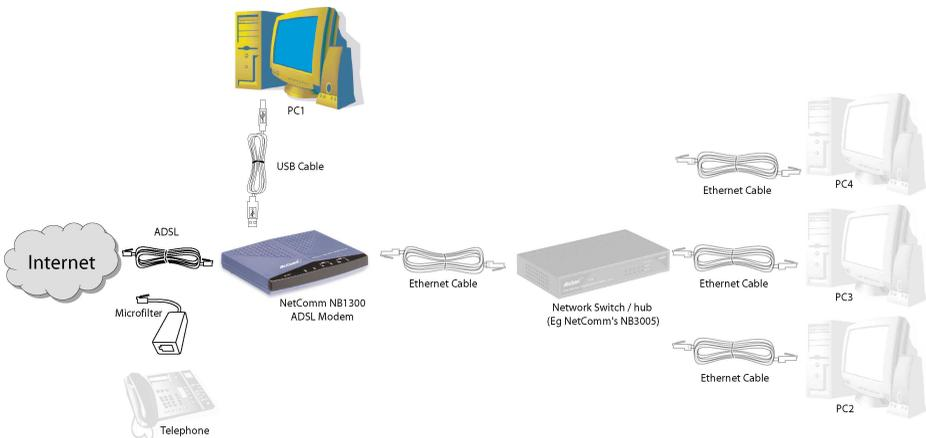
**USB Gateway Configuration** (Multiple public IPs to Multiple internal IPs) - If you do not have an Ethernet port on your computer you can use your USB port like an Ethernet port to connect to the NB1300. This "simulated" Ethernet port is only for connecting to the NB1300 and is only available for Windows 98SE, Windows 2000 and Windows XP. The NB1300 will log on to your ISP on behalf of your computer and it will shield your computer from Internet attack by using NAT.
