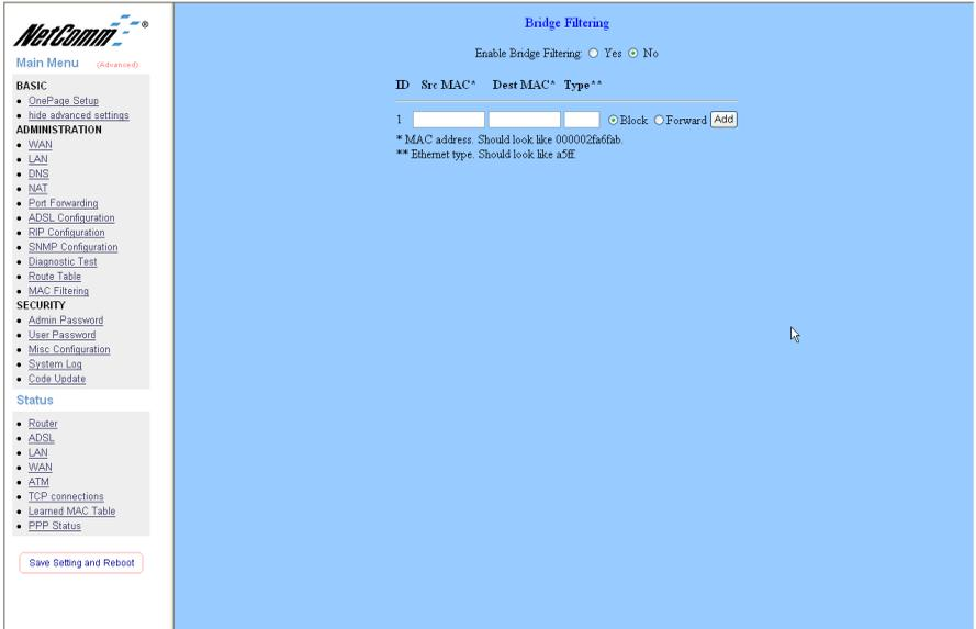
**Source MAC:** When the bridge filtering is enabled, enter the Source MAC address, select Block and click Add. Then all incoming WAN and LAN Ethernet packets matched with this source MAC address will be filtered out. If the Forward is selected, then the packets will be forwarded to the destination PC.
