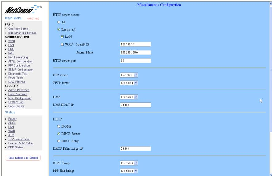
**HTTP Server Access:** This field allows the user to configure the Web pages can be accessed from.
