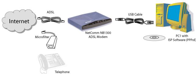
**ADSL modem** (Transparent Bridge) to be connected to a router - This is when you plug the modem directly into the USB port of just one computer. You then must run Internet connection software (often supplied by your ISP) on the computer to establish a connection to the Internet. This method means that the computer connected to the USB port of the NB1300 is exposed to the Internet and is given a public IP address.
