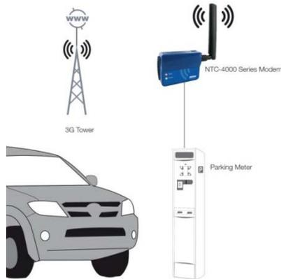
Figure 37 - Parking Meter Deployment
