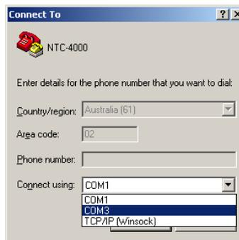
Figure 19 - NTC-4908 Operation Settings - Select COM Port
