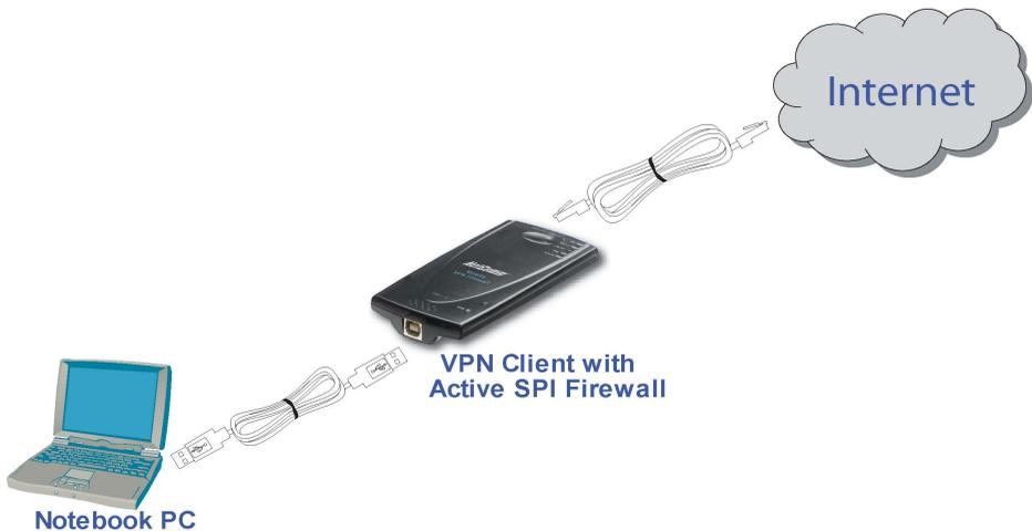
3. Connect one end of an Ethernet cable to the Ethernet port on the Adapter, and the other end to an Ethernet port (LAN port) on a Network. If you are not using a Router, you can connect it directly to a Cable or DSL modem.
