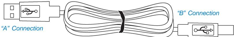
By using different connectors on the upstream and downstream ends, cable connection is simplified. The "B" connection will fit into the "B" socket of any USB device. Similarly, any "A" connector can be plugged into any "A" socket, such as on a computer.
