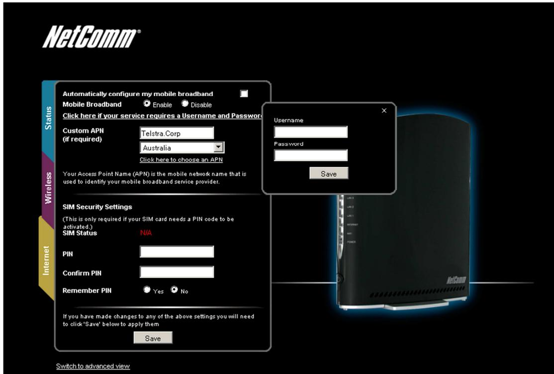
Figure 5: Basic View - Internet – Telstra IPWAN Setup
