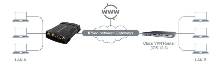
Figure 3 – M2M router to Cisco VPN router Site-to-Site network diagram and policy planning
