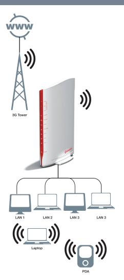
The HSPA+ WiFi Router offers unparalleled speed and coverage over a 3G HSPA+ network. With a peak downlink speed of up to 21Mbps and uplink speed of up to 5.76Mbps, this device will have you accessing a mobile broadband connection with speeds equivalent to those of a fixed ADSL broadband connection.
