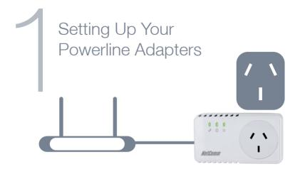
Using one of the supplied Ethernet cables connect one end into the LAN Ethernet port of your modem/router.
