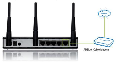
2. Connect all your computers, network devices (network-enabled consumer devices other than computers, like game console, or switch / hub) to the LAN ports (1-4) of the router.
