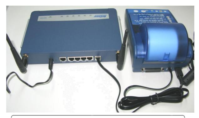
Connect the HS1100/IAC3000 to the AG400 Thermal Ticket Printer via the RJ11 cable provided.
