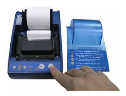
Remove the cover, then insert the paper roll and press "LF" to let the paper be drawn into the print mechanism. Then close the cover.
