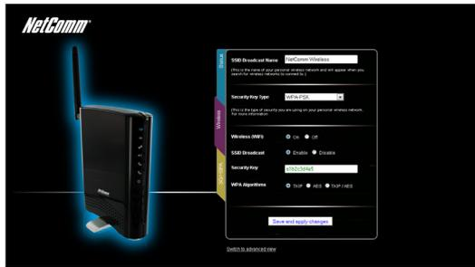
This page allows you to configure basic WiFi settings for this device such as enabling/disabling the WiFi functionality, changing the Wireless Network Name (SSID) and Wireless Security settings.
