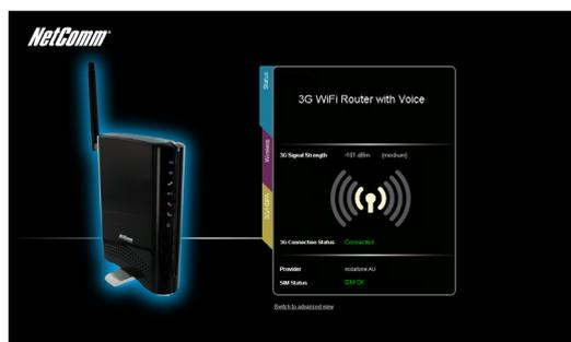
The status page shows the 3G connection status, Signal Strength (dBm) and SIM Status.
