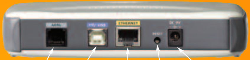
RJ11 for ADSL connection to telephone line USB data port RJ45 Port for 10/100 Ethernet LAN connection Reset/factory defaults Power jack for AC power adaptor USB/RJ45 ports can be used simultaneously
