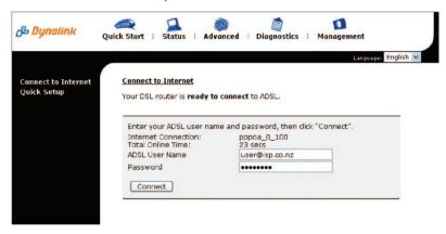
Once connected the screen changes to display the on-line time. The PPP light on the front panel of the router will come on, indicating that you are online. Click **Disconnect** only if you wish to disconnect manually.
