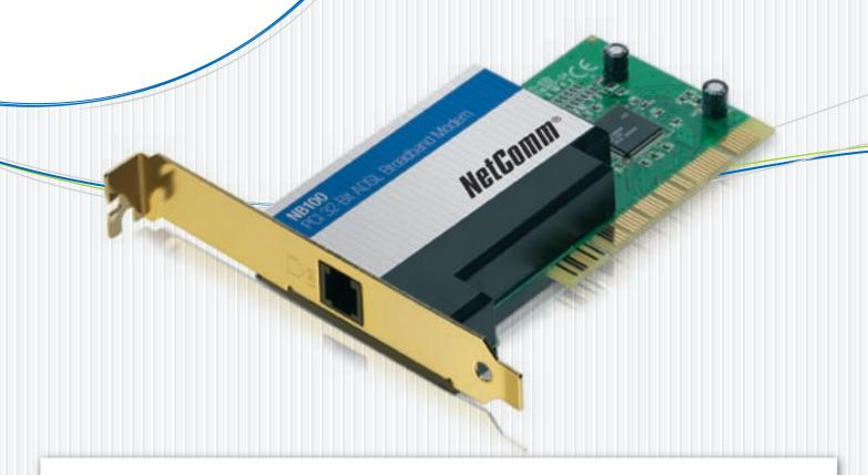
The **NetComm NB100** is a PCI 2.3 standard compliant ADSL modem device that provides an "always on" high speed broadband connection to the Internet. Fully compliant with ANSI T1.413 Issue 2, ITU G.992.1 and ITU G.992.2 standards, the NB100 – with data tansfer rates of up to 8Mbps downstream and 1Mbps upstream – is the ideal solution for high-bandwidth applications such as access to a corporate network, internet and video.
