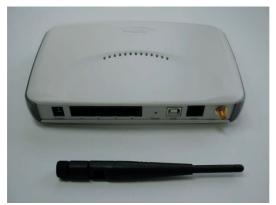
Note: Your equipment must have a detachable SMA antenna in order to use the NP56o/NP562 NetComm Wireless Booster
