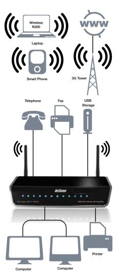
The NetComm 3G10WV integrates a Wireless LAN, HSPA module and voice gateway into one stylish unit. Insert an active HSPA SIM card into the slot on the rear panel and get instant access to a 3G Internet connection.
