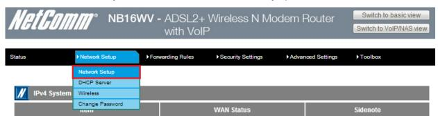
4. Select the **Wireless WAN** as the WAN Interface. The Wireless WAN option makes use of the mobile broadband dongle connected to the NB16WV.
