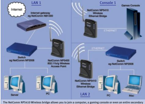
Wired Network (LAN 2) to an existing Wireless network (WLAN). If your existing Wireless network has access to the Internet or a Primary Wired Network (LAN 1) then these will also be available to devices connected to the bridge.
