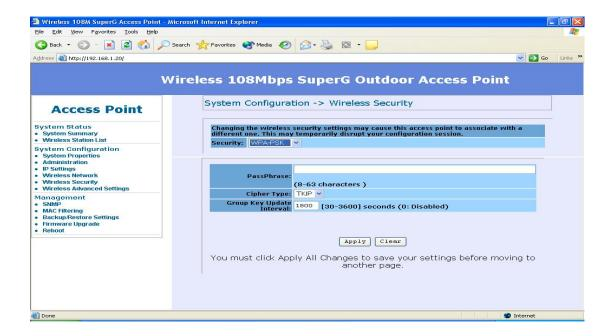
WPA option features WPA used in coordination with a RADIUS server. (This should only be used when a RADIUS server is connected to the Access Point.)
