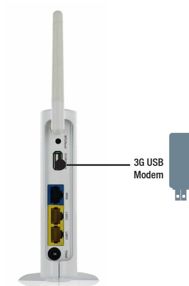
Note: The 3G17Wn - 3G Wireless N150 Router is designed to work with 3G USB Dongles that can be used as data modems (support tethered data). Please refer to your service provider for detailed feature information. Please refer to the NetComm website for a list of compatible 3G USB Modems
