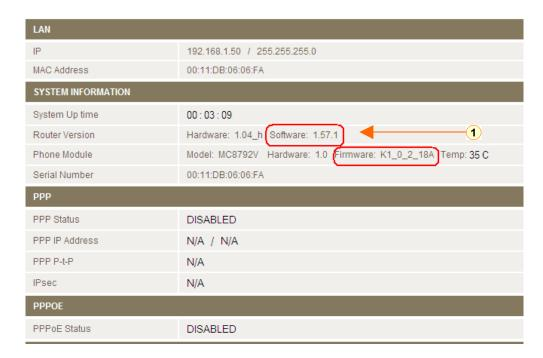
You will notice that the NTC-990 is running phone module firmware version K1\_0\_2\_18A.
