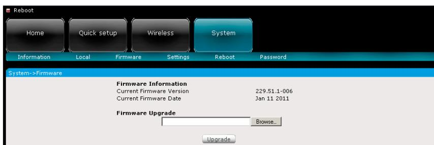
The firmware page allows you to see the current firmware version and build date as well as upgrade the firmware running on the NP124.
