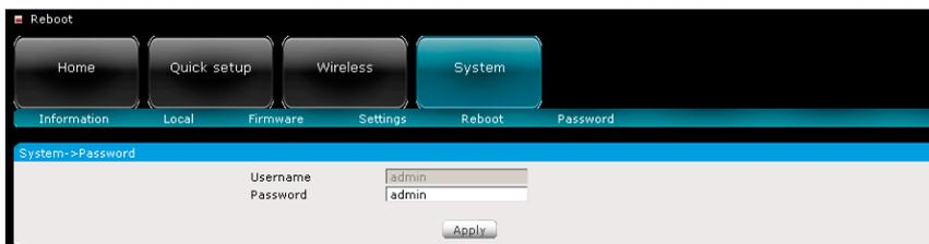
The password page enables you to change the password required to access the web based configuration pages.
