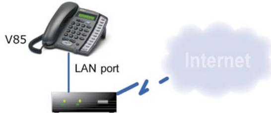
ADSL Modem or router in bridge mode
