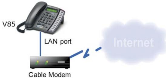
Alternative V85 connection type with Cable Modem
