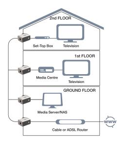
NetComm's Powerline Adapters harness the potential of Ethernet-over-powerline technology to give you the ability to network your home or small business using the existing electrical wiring, without the setup problems and coverage gaps associated with wireless devices.
