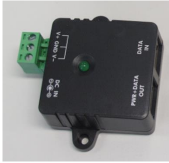
Figure 11 - Assembly of the PoE Injector and the Captive Terminal Block
