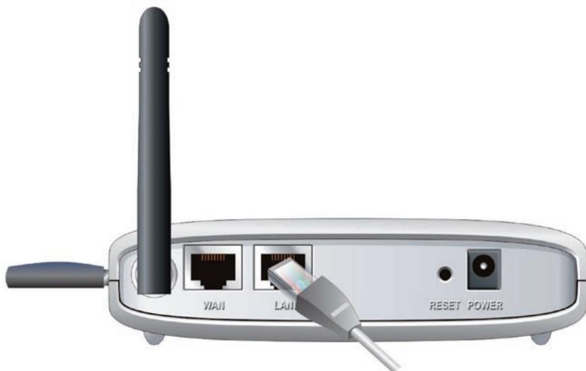
*Note: The N3G001W 3G Wireless Router LAN Port is "Auto-MDI/MDIX." This provides Ethernet cable LAN Port access.*
