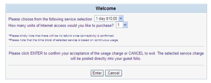
Click the *Enter* button to accept the charge. This information will be sent to the PMS system via the console port on the rear of the IAC4000.
