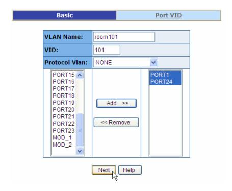
Packets traveling into PORT1 are *untagged* and packets traveling into PORT24 need to be *tagged* before they are sent to the IAC4000. Click *Apply* once done:
