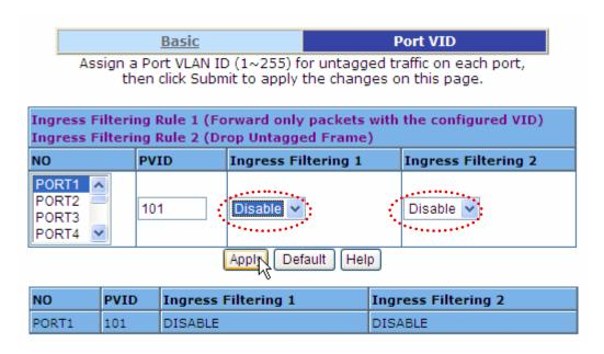
Select PORT24. Disable Ingress Filtering 1 and Ingress Filtering 2. Click Apply:
