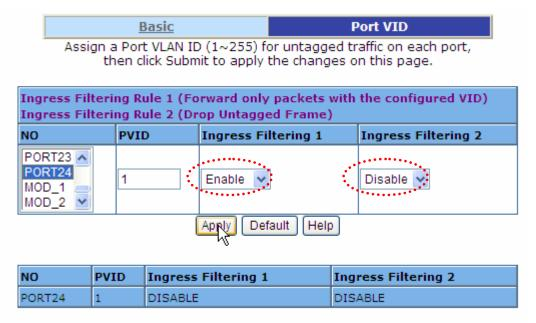
Configure other ports and reboot the NP2624M for settings to take effect. Then connect Port24 of the NP2624M to one of the LAN ports on the IAC4000.
